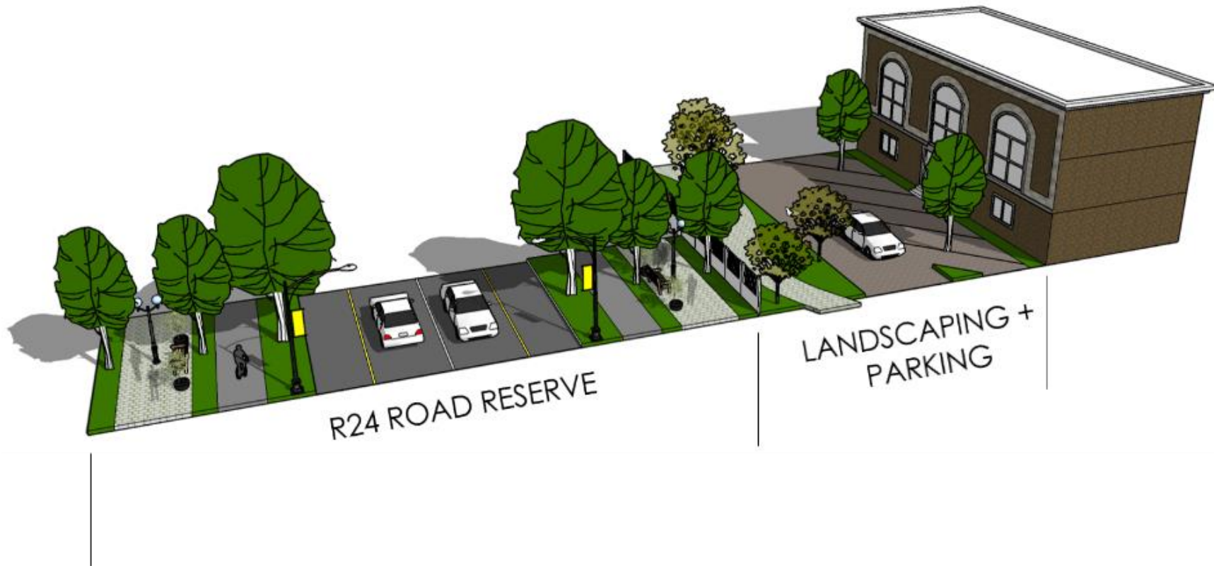
Figure 49: R24 STREET SECTION
